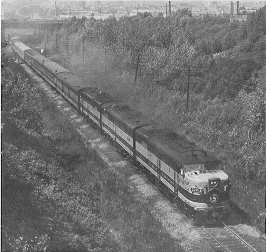
A trio of Alco cabs exits Vancouver through the 1.1% "cut" with the Afternoon International in tow.
