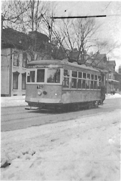
LEFT: The discussion vis-a-vis air brakes on single-truck cars was solved by the appearance of the Birney safety car. No. 129 of the Halifax system is shown, 1939.
