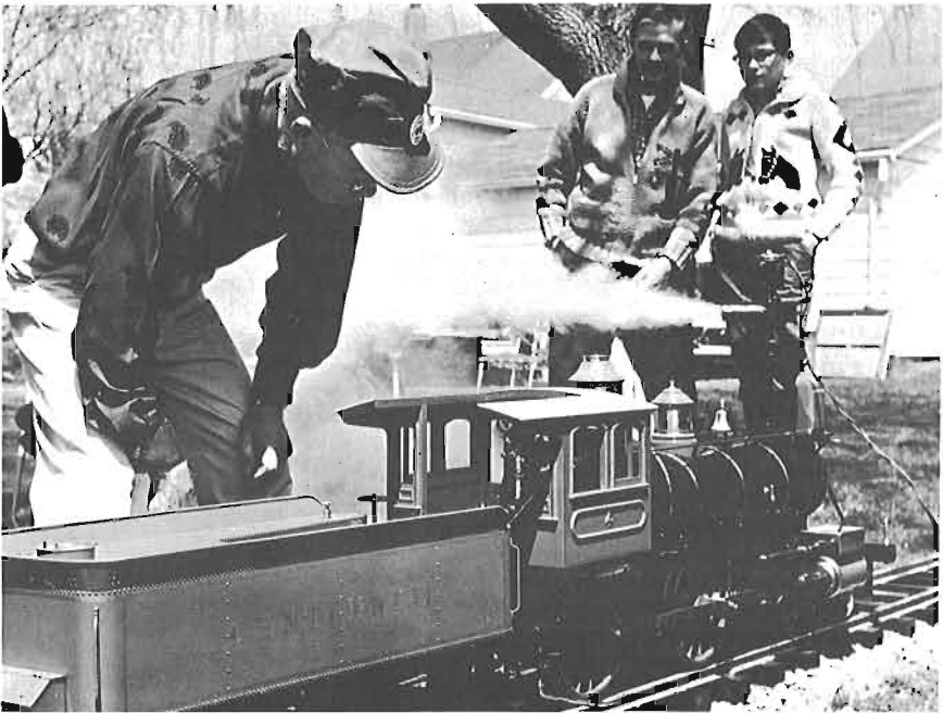
Harry C. Allin, Etobicoke, checks the steam pressure as he fires up his personal Centennial project. The 7 1/4" gauge "Centennial #4" is a precision model of a locomotive that hauled trains from Aurora to Toronto at the time of Confederation. Mr. Allin built the coal-fired model in 1500 working hours and gave it its Centennial run May 13 at a garden ceremony for the Toronto Society of Model Engineers.
