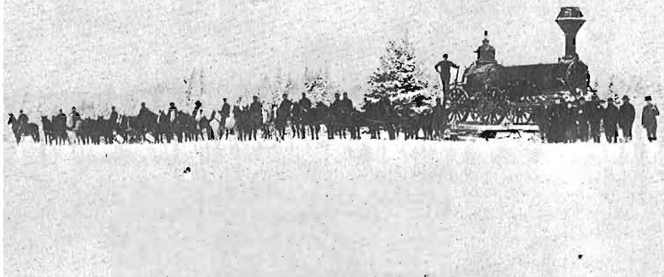
PHOTO ABOVE: Last ride of the locomotive No. 1 "HERCULES". Built by Hinkley of Boston in 1854, she later became Intercolonial No. 1. Photo taken near Point du Chene N.B. engine being transported to Bateman's Brook for use as a sawmill stationary boiler:
