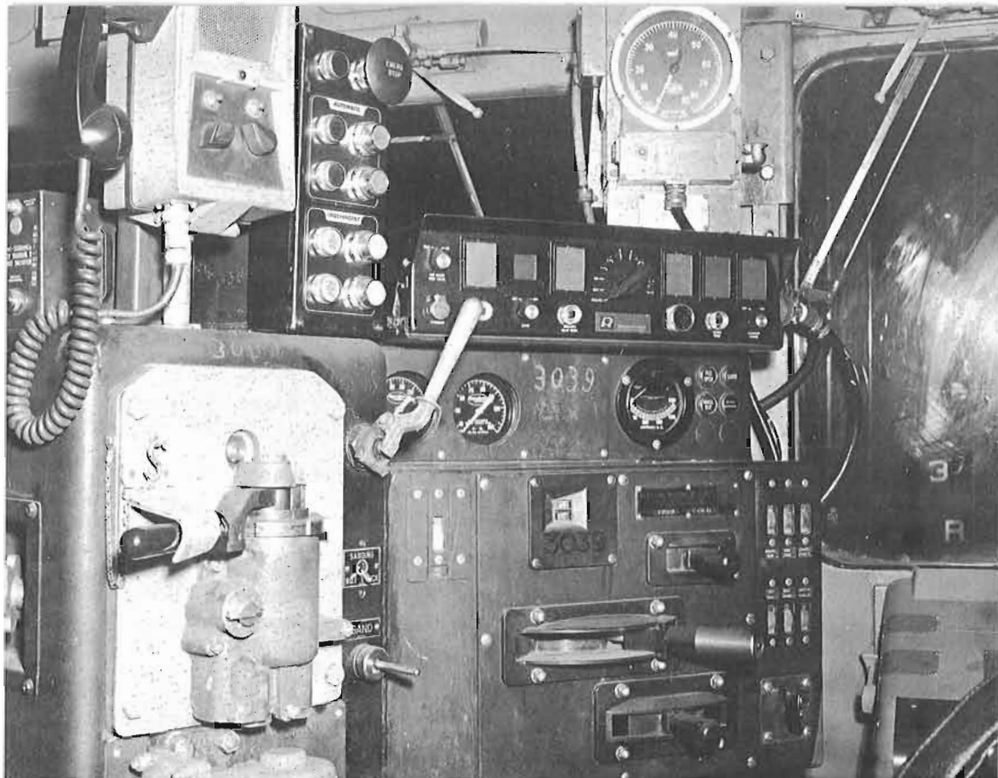
↑ THE CONTROL POSITION IN THE MASTER CONTROL UNIT. All of the accessories necessary to the control of head-end and slave units are provided on or near the unit control panel. Photo Radiation, Incorporated.
