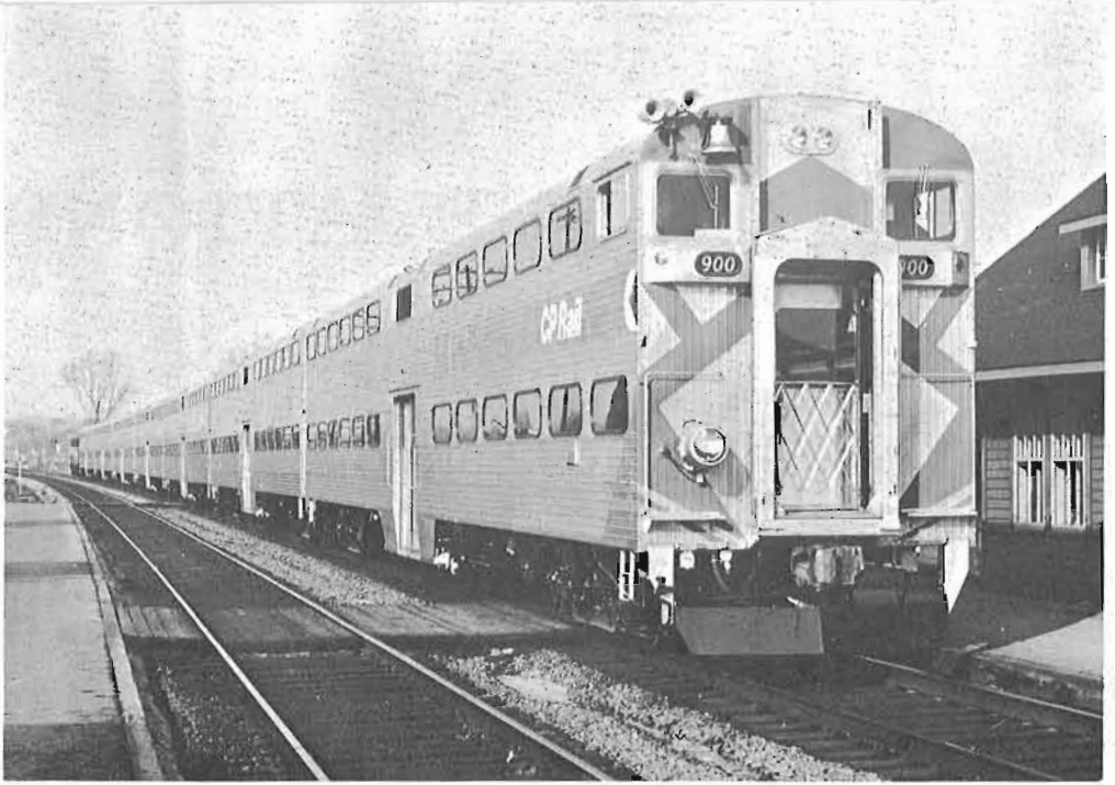
A COMPLETE TRAIN OF GALLERY CARS, HEADED BY CONTROL CAR NO. 900. JUST Visible at the rear of the train is the diesel unit supplying the power. Photo courtesy of R. Ian Stronach.
