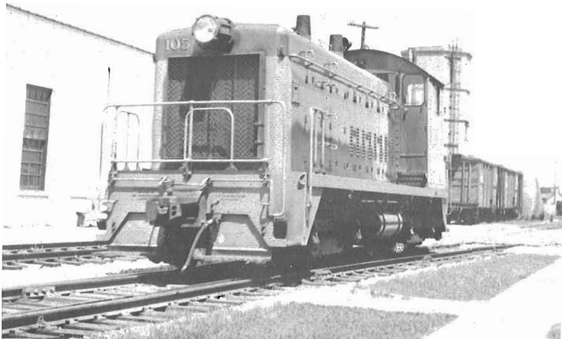
↑ ESSEX TERMINAL RAILWAY'S 1200 HP. GMDL SW1200 NO.105 - BUILT 1956 - BESIDE the engine house at Windsor,Ontario. Just beyond the boxcars is the ETRy's 0-6-0 steam switcher,swathed in tarpaulins - outside to provide space inside for the diesel switchers. Colour scheme is green with yellow running boards and panels on each side of front radiator. Photo courtesy W.J.Redbrook.
