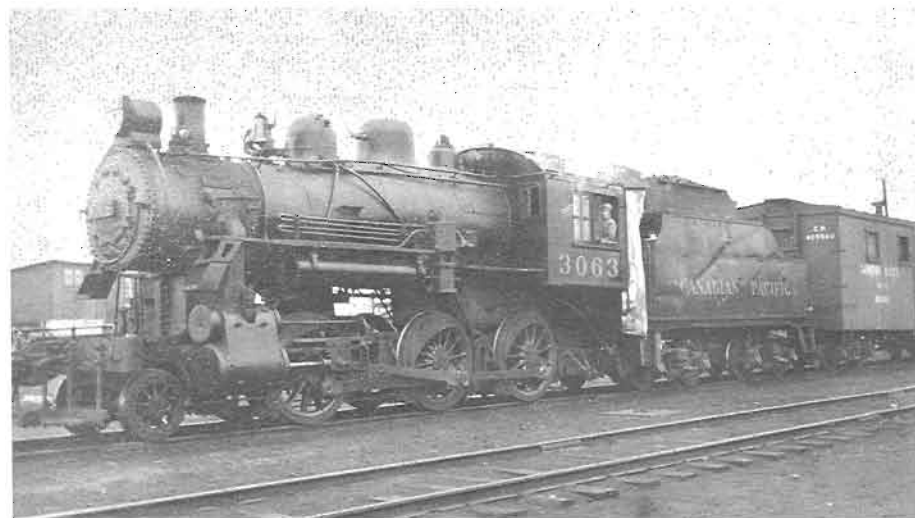
A PRAIRIE TYPE 2-6-0 ENGINE NO.3029 OF CANADIAN Pacific Railway. Photo courtesy Canadian Pacific. ANOTHER VARIETY OF THE PRAIRIE TYPE - NO. 3063 of Canadian Pacific photographed at Smiths Falls, Ontario on March 18, 1947. Photo coll. L.O. Leach.
