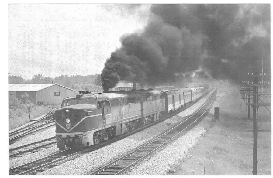
in air volume, thus achieving complete, smoke-free combustion. If this were possible, there would be no smoke or incompletely-burned fuel particles from the exhaust stacks.
