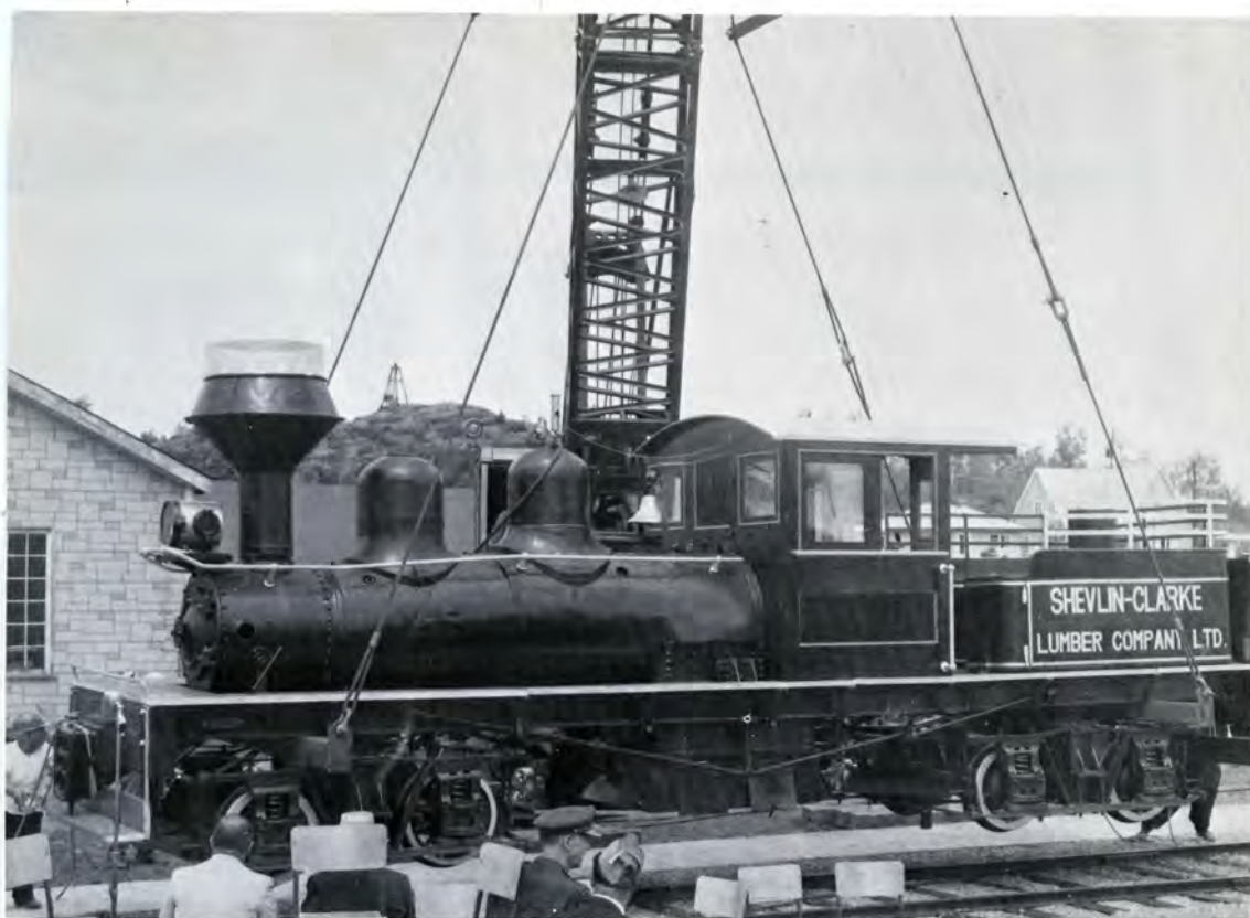
↑ WITH THE AID OF A CRANE, SHEVLIN-CLARKE LUMBER COMPANY'S TWO-TRUCK Shay locomotive is lowered onto the "podium" in Atikokan's Civic Centre on 6 July 1963, the realization of Mr. W.S.Peruniak's "better idea". Photo courtesy W.J.Bedbrook.
