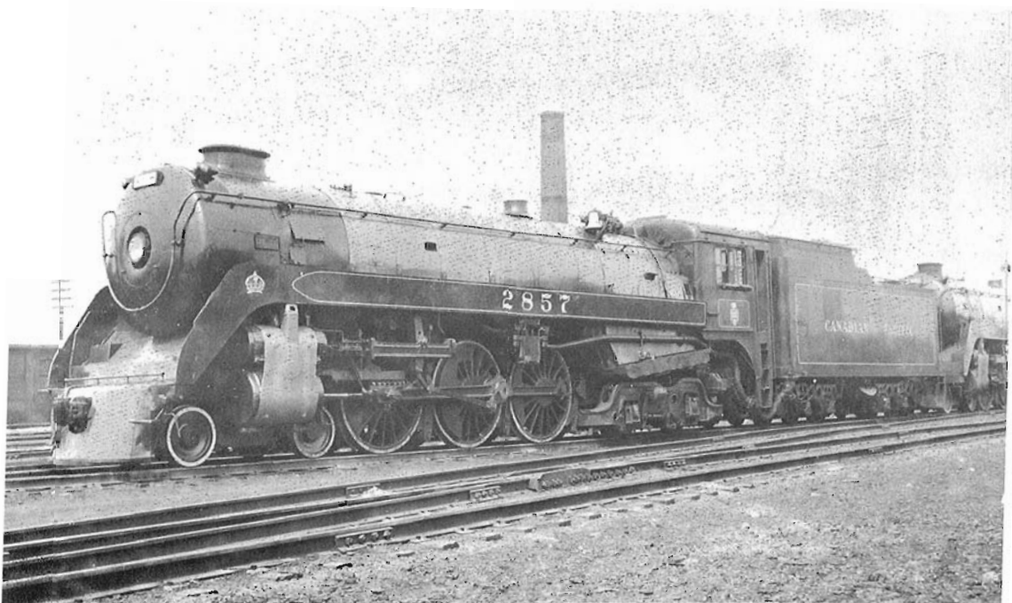
A BEAUTIFUL EXAMPLE OF A "ROYAL HUDSON" H-5-d CLASS, CANADIAN PACIFIC Number 2857, was photographed at West Toronto in April 1959. This locomotive was built by Montréal Locomotive Works in 1938.
