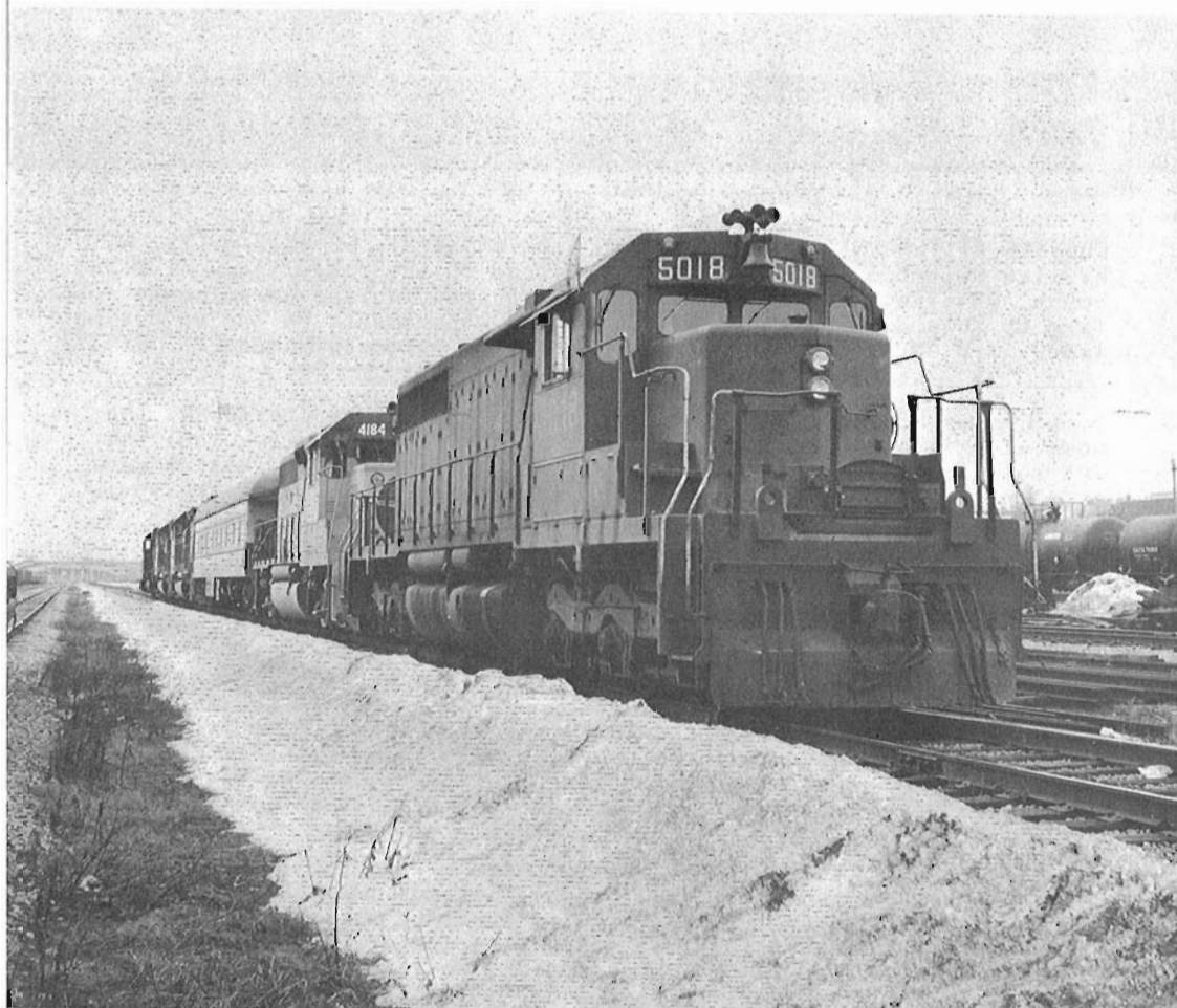
CANADIAN NATIONAL RAILWAYS UNIT NUMBER 5018, CLASS GF 30, BEING TESTED with Chessie System unit Number 4184, with British Columbia Railway unit Number 69, Chessie System units Numbers 4181 and 4182 and Canadian National unit Number 2007 providing the dynamic brake load. The test was conducted on Track 029, Turcot Yard, Montréal, on March 14, 1973.
