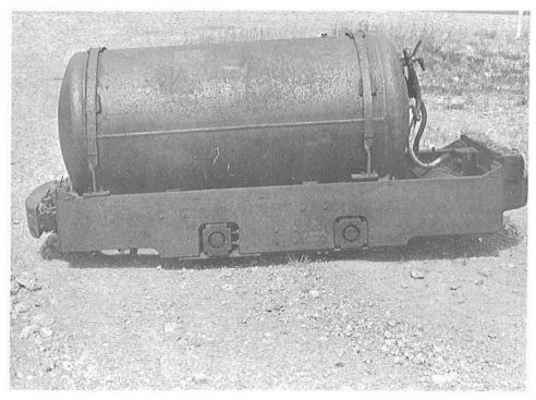
CANMORE MINES LIMITED GENERAL ELECTRIC LOCOMOTIVE NUMBER 1 DRAWS ITS power through an overhead "slider" trolley. It was built in April, 1952.
