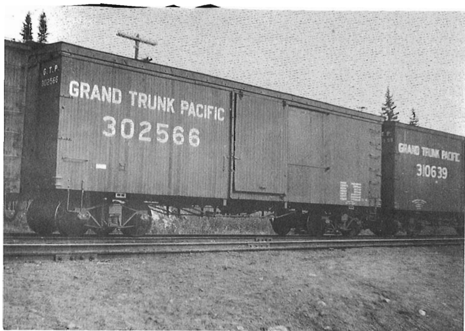
A GRAND TRUNK PACIFIC BOXCAR OF THE TURN OF THE CENTURY, COMPLETE with truss-rods and arch-bar trucks, recorded at Dona, Ontario, by T. Delvecchio.
