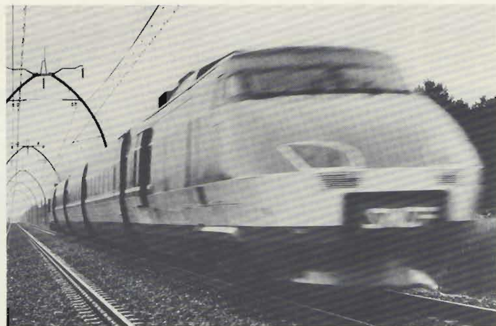
IN 1973, THE TGV-TYPE TURBOTRAIN OF THE FRENCH NATIONAL RAILWAYS RAN at more than 300 km per hour between Bordeaux and Irun in western France, over long sections of welded rail on concrete ties, with double elastic tie-clips. Photo courtesy French National Railways.
