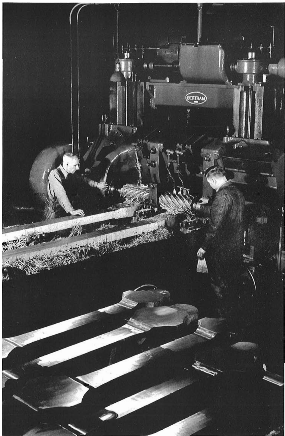
Proof positive that steam locomotives were built at Angus as we witness here the milling of a pair of main rods in 1948.
