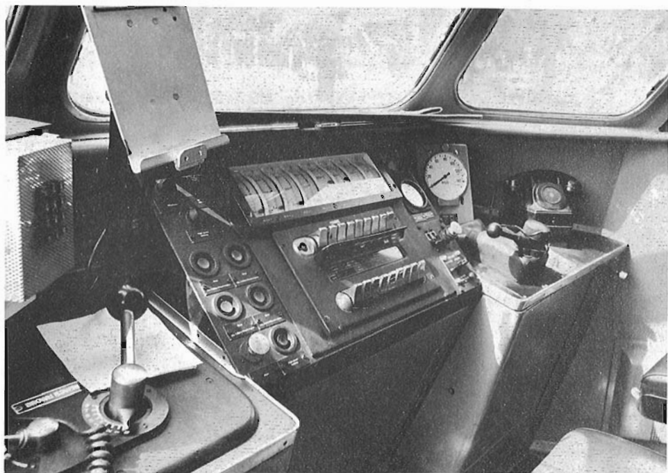
An engineers eye view of the compact yet modern control console. All indications appear to be in the metric system probably making the train a forerunner of this system of measurement which is presently being introduced nationally.
