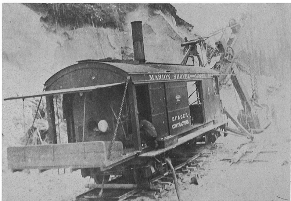
Marion Steam Shovel ' model 60 ' as used by E.F. and G.E. Faquier contractors on the construction of the National Transcontinental Railway in the Nipigon region. T.S.Armstrong photo.
