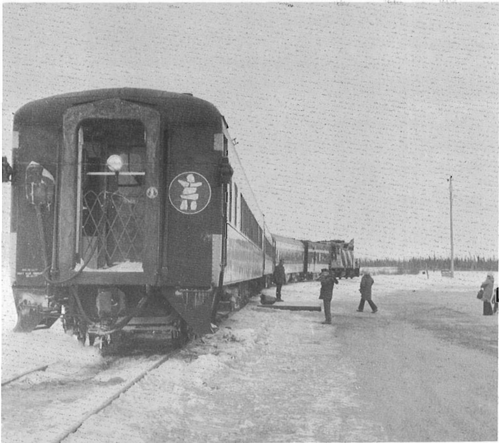
Tail end view at Pine Point, N.W.T., note the special reversing headlight to provide illumination during the reverse moves required. All photos courtesy Mr. Peter Lofthouse of Yellowknife, Northwest Territories.
