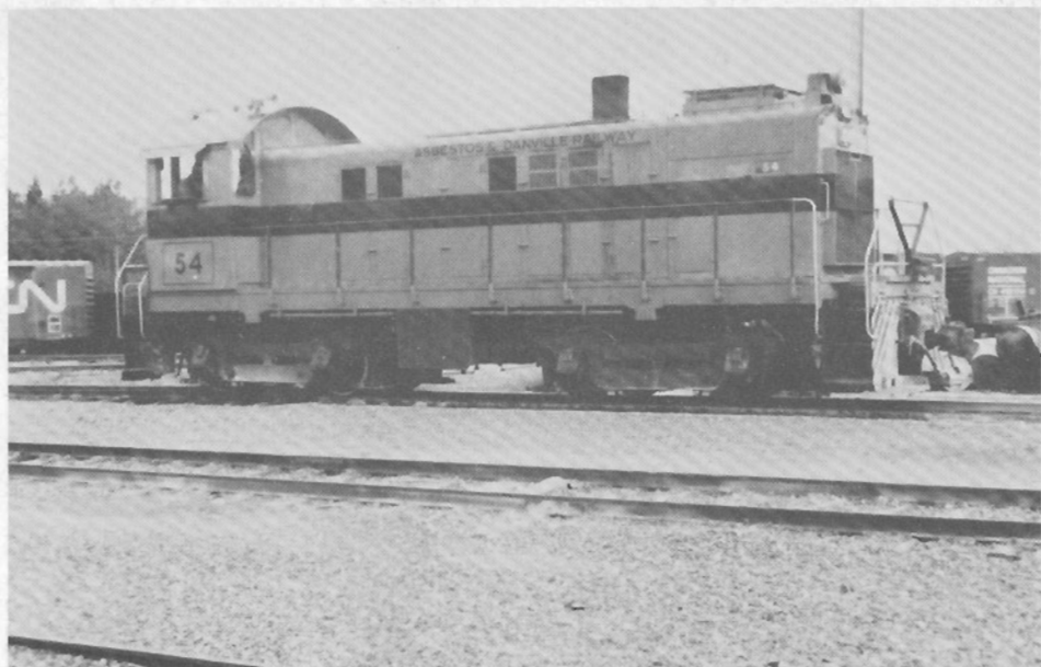
The Asbestos and Danville Railway has purchased 3 Southern Pacific Alco S-6's rated at 1000HP each. Pictured is No. 54 believed to be ex SP 1238, serial 81812. The photograph was taken at Asbestos, Quebec on 16 September, 1977.
