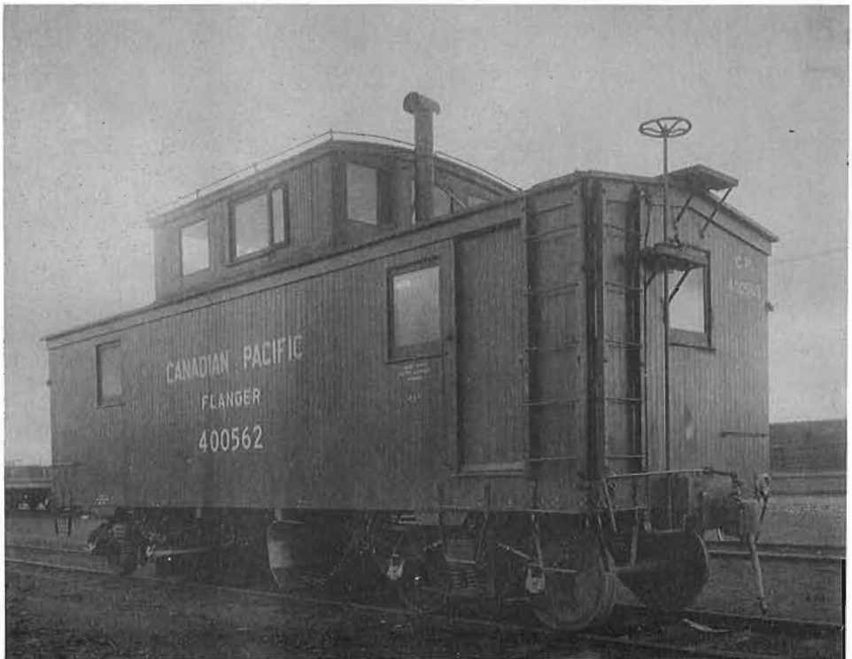
A fine example of a wooden flanger immediately after construction at Angus Shops, Montreal in 1913. Two sets of flangers beneath the car permit double ended operation.
