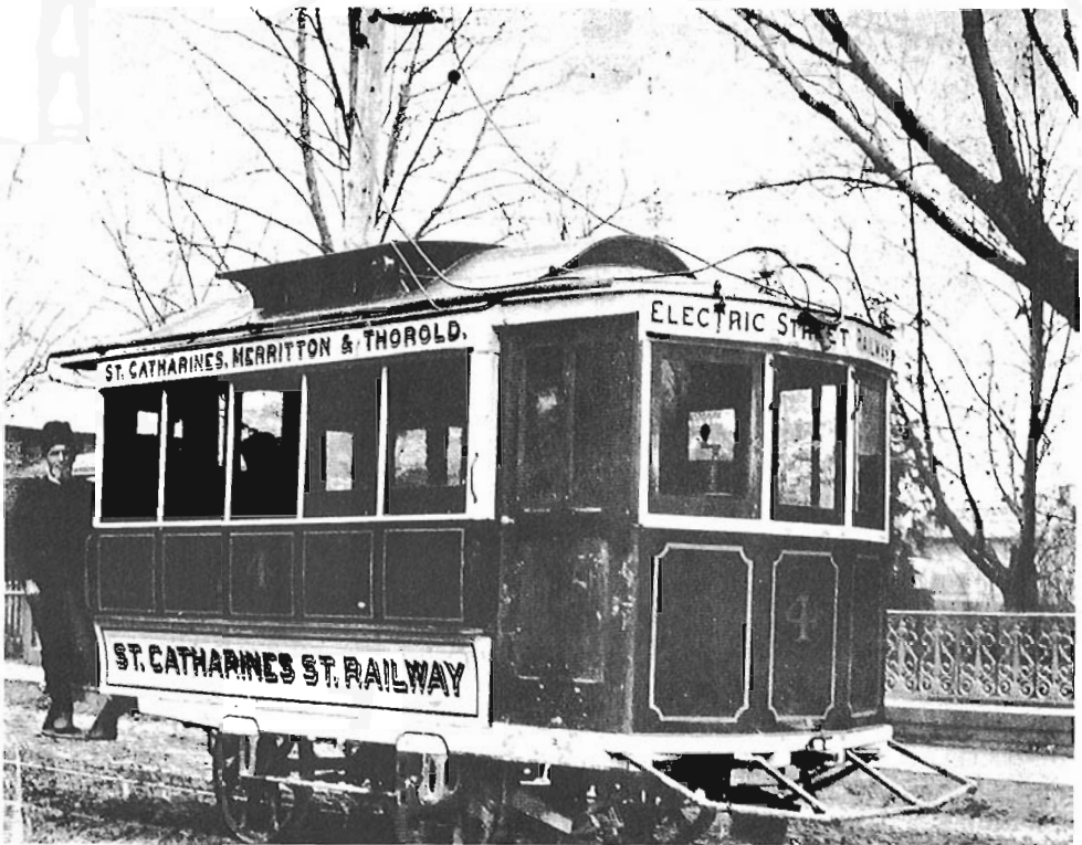
The St. Catharines Merritton and Thorold was one of the first electric railways in permanent operation in Canada. Here is one of their first electric cars, obviously a converted horse car, photographed in 1887. (Trolley Car Treasury)
