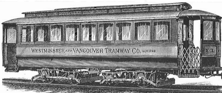
Twenty-five Feet Vestibuled Car Body Mounted on Brill's Eureka-Maximum Traction Trucks.
