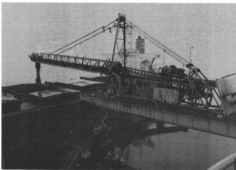
The conveyor gantry and delivery tube is shown in position above open hatchway of ocean carrier.
