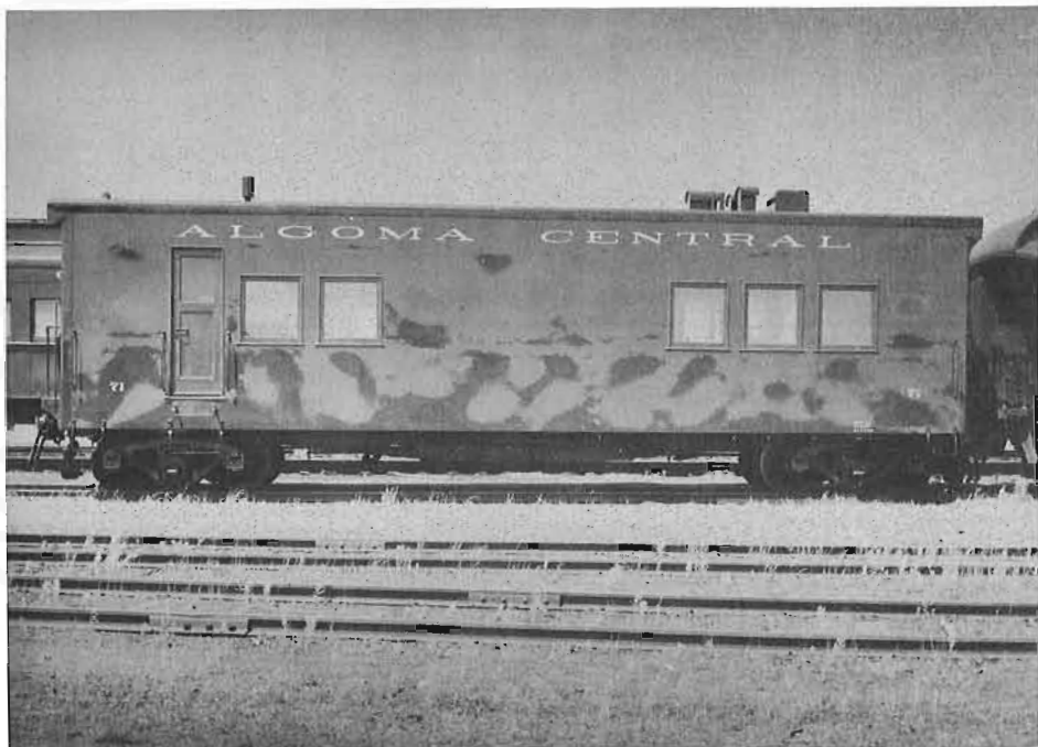
One of the homebuilt steam generator cars as it looked in 1952. These were in addition to the troop sleeper conversions. RPS photo from the Author's Collection.
