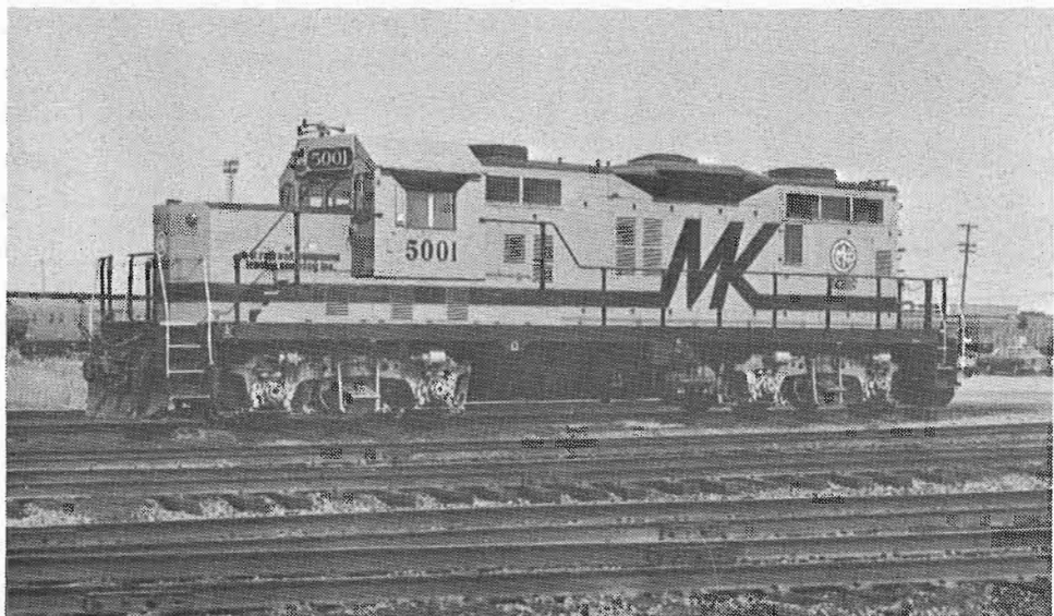
MORRISON - KNUDSEN 5001 is ex - U.P. GP-9 No. 278 fitted with a 6-cylinder prime mover instead of the EMD 16-567C. Pictured on July 5 1980 while at St. Luc yard.
