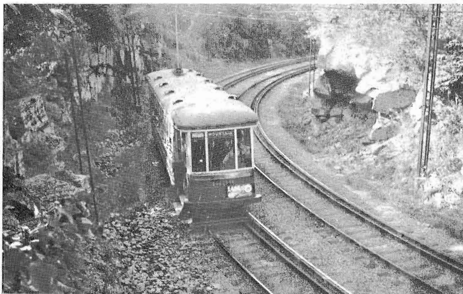
No. 1339 ROUNDS THE ROCKY CURVE just before starting the straight ten percent climb towards the Eastern portal of the tunnel. This car, built in 1913, is now preserved at the Canadian Railway Museum, where it represents not only the Mountain route, but also the largest class of street cars ever to run in Montreal. Collection of R.M. Binns.
