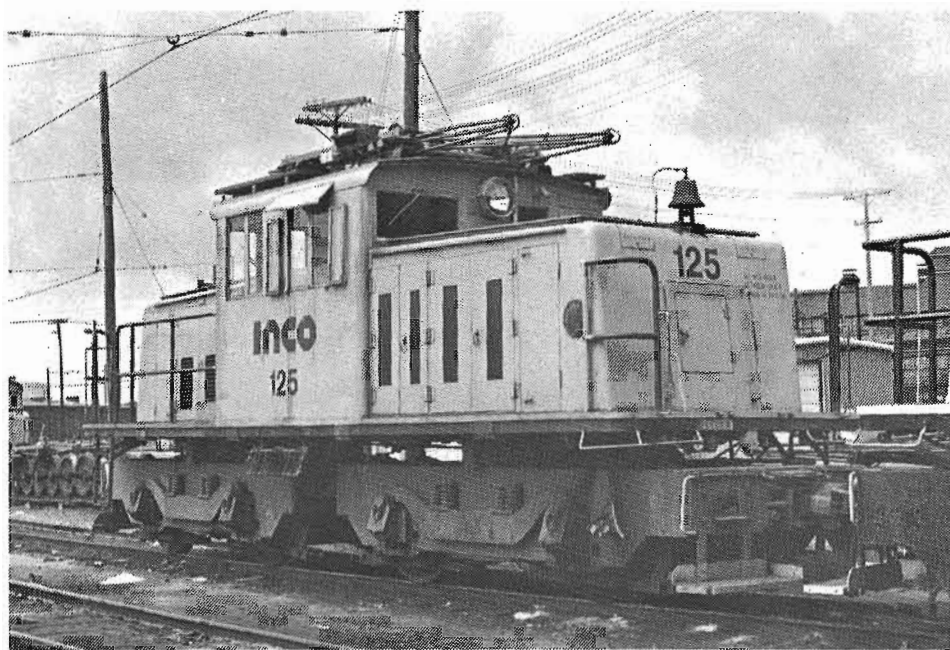
INCO Railway No. 125, a G.E. 85-ton electric locomotive built in 1950.
