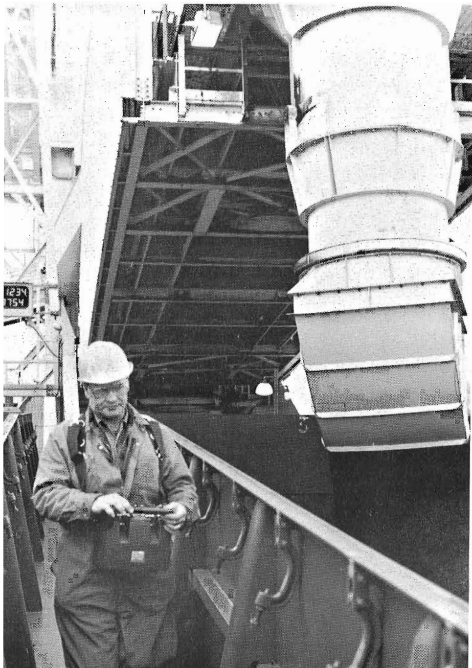
ON BOARD THE "CANADIAN TRANSPORT". The "Shiploader" is radio controlled by the foreman on board the ship. Note the sign in the left background showing 19,754 tons loaded so far. Kenneth A.W. Gansel, June 1980.
