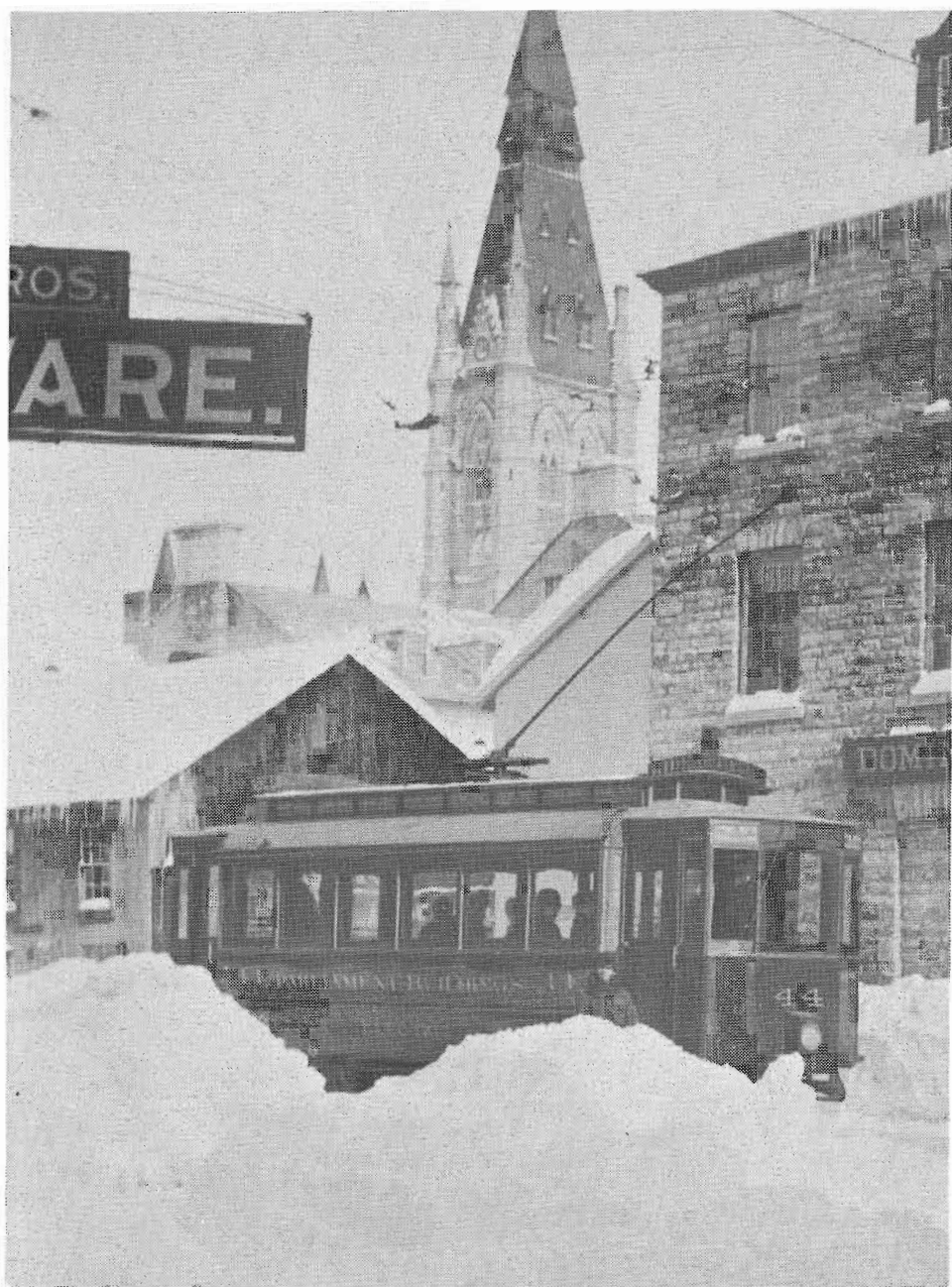
IN THE SHADOW OF THE PARLIAMENT BUILDINGS Ottawa Electric Railway car 44 makes its way along a snow-covered street in the early 1890's. This car was one of the earliest built with permanent vestibules, and cars of this type (all built by Ottawa) were used in several Canadian cities in the 1890's.
