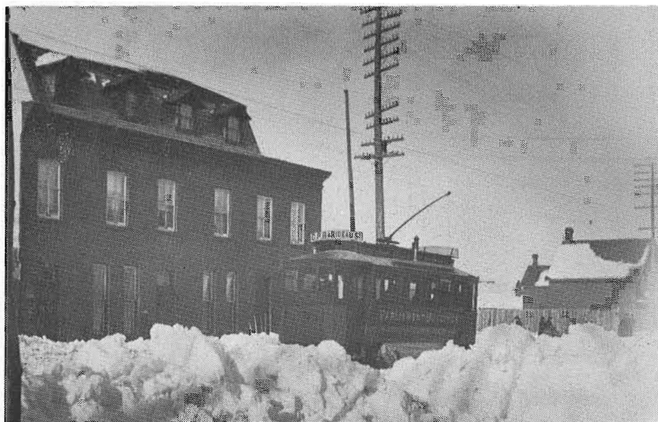
ANOTHER EARLY OTTAWA CAR, No. 17 surrounded by snow banks about 1892. This is one of the earlier cars which has had the vestibules added, probably the first winter. Note the canvas hung at the side to protect the motors from slush.
