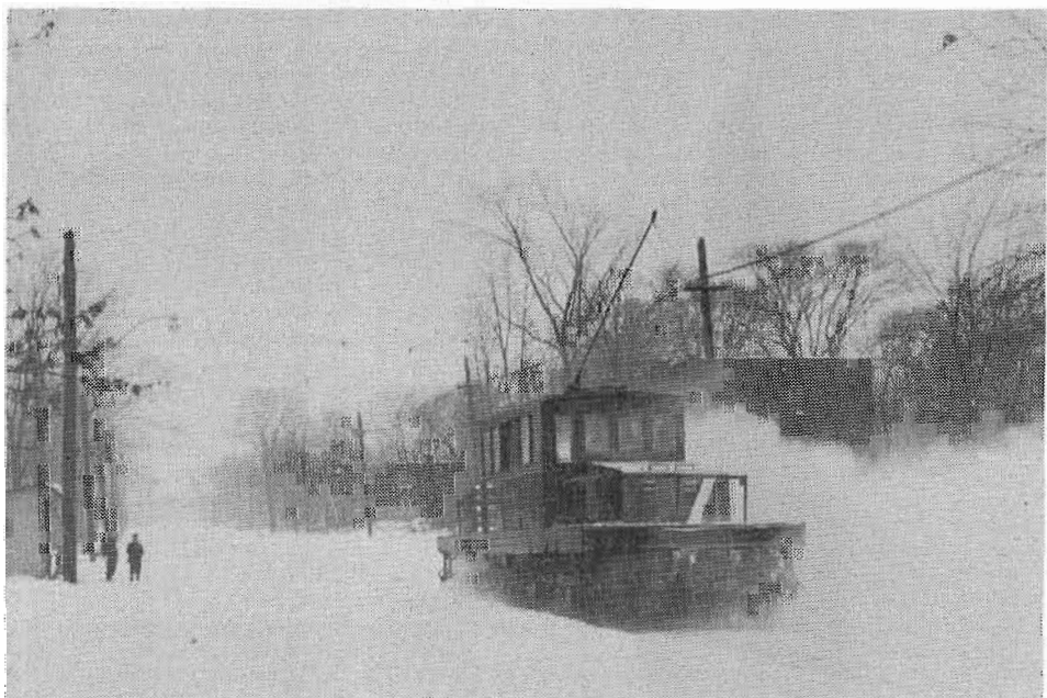
THE MONTREAL AND SOUTHERN COUNTIES RAILWAY is usually remembered for its interurban lines; however they also had the line to Montreal South which ran on city streets. These two photos were taken on Jan. 6 1951, and show sweeper 303 busily at work on Desaulniers Blvd. in St. Lambert. Toohey Collection, C.R.H.A.
