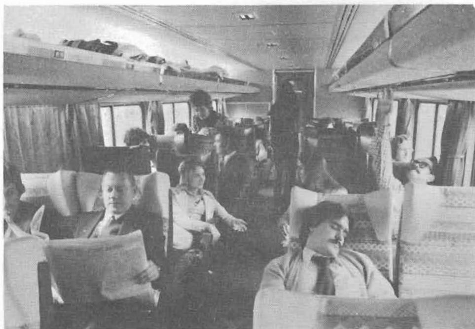
Amtrak's Superliner coaches make long-distance rail travel most comfortable. Built by Pullman Standard, the bi-level cars seat 77 passengers with 62 on the upper level, 15 on the lower. Each of the reclining seats features arm and leg rests, individual reading lights, attendant call buttons and fold-down tray tables. (Amtrak Photo)
