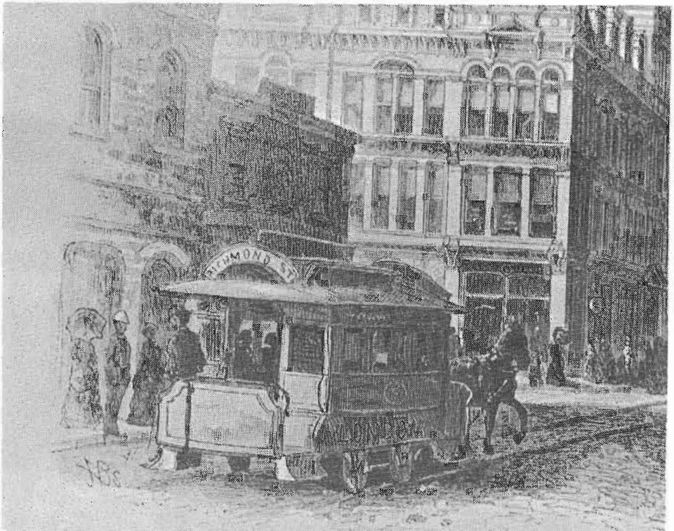
A HORSE CAR ON RICHMOND STREET IN LONDON ONTARIO in 1882. This is typical of the thousands of horse cars that provided the bulk of transit service in most of the cities of North America in the 1880's. Where there were steeper grades two horses would be used.
