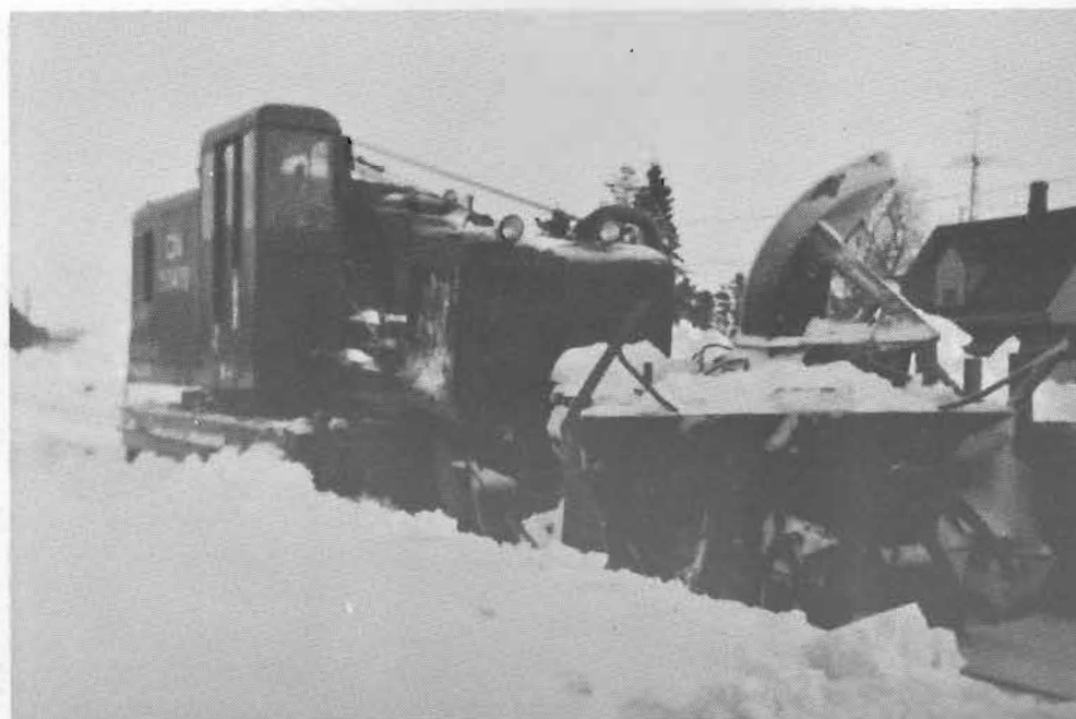
A FRONT VIEW OF THE SNOW BLOWER ATTACHMENT on a C.N. crane which was able to clear the line right to Tignish.
