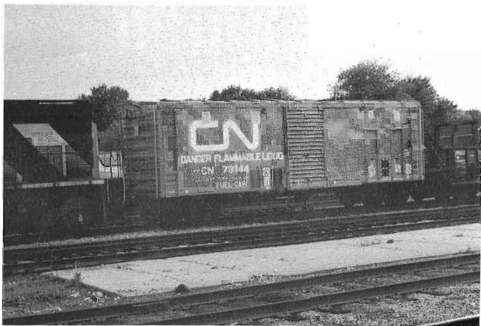
C.N. FUEL CAR 73144 at Stratford on May 29 1982. This car is painted bright orange and is used in work train service,
