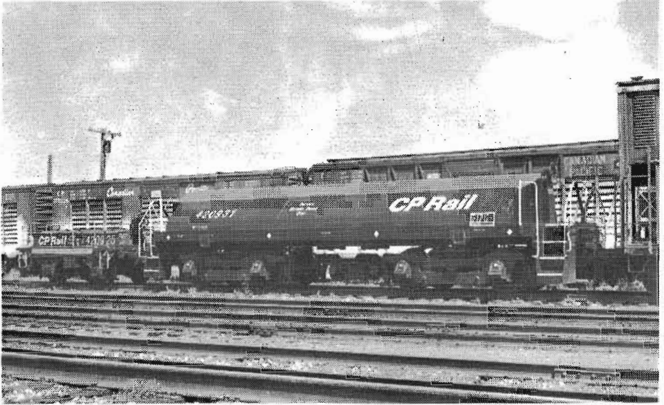
SCALE TEST CAR 420931 was built on the frame of a scrapped switch engine at West Winnipeg shops in April 1982. Curiously it has one Canfor and one Dofasco truck. Apparently it was doing comparison tests when photographed here at Brandon as regular car 420925 was travelling with it.
