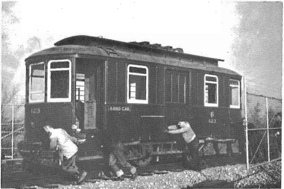
FORMER OTTAWA MAIL CAR 423 being moved through the gate on December 1 1962. Once the momentum was established it was fairly easy to move a street car due to the inertia of the rotating armatures which acted as a flywheel to help it over the hard spots.
