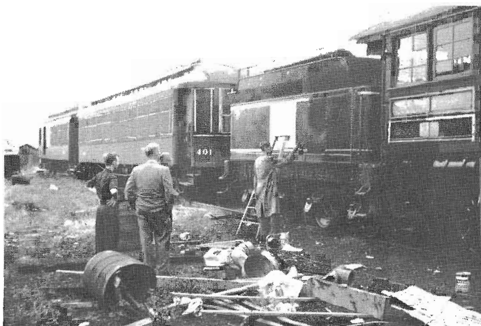
RESTORATION WORK BEGAN even before the equipment was moved to the museum site. In the creosoting yard on August 20 1962 Maritime Railway No. 5 was cleaned and painted. Here we see Peter Murphy spraying the tender while Donald Angus, Robert Halfyard and Bruce Millar look on.
