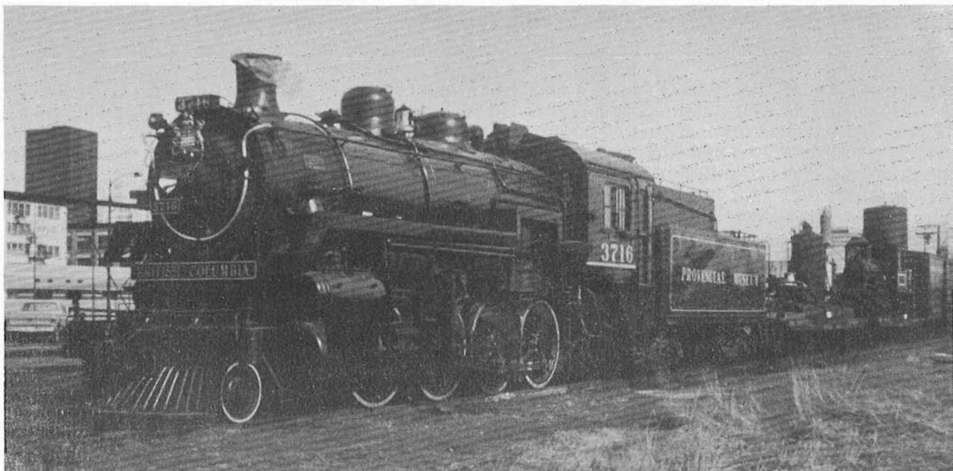
B.C. Museum Train, Drake St. Yard #3716 a Consolidation freight engine 2-8-0 built in 1912, shown in off-season rest.
