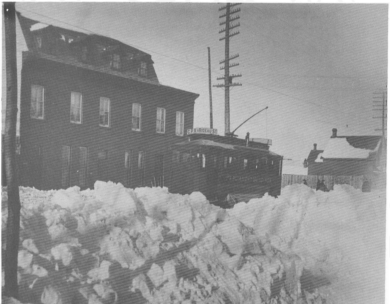
Ottawa Electric Railway street car No. 17 on a snowy street in 1892. This is one of the earliest electric cars, it was built with open platforms but had vestibules added for winter use. After 1891 all closed cars were built with permanent vestibules. This photo is also rare in that it is the only one seen of an Ottawa passenger street car with a number containing the digit "7". At some early date, for reasons now unclear, the company stopped using any numbers that contained seven.
