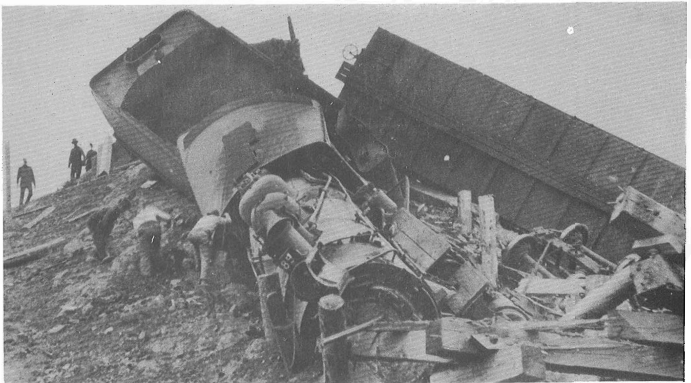
Long before the age when block signals would have protected him, and driving into heavy rain, the engineer of the 851, a heavy 2-8-0 on an eastbound freight train, had no warning of impending disaster until the track disappeared under his headlight beam. The resulting wreck was fatal for the three man crew on the engine. Some area residents will tell you the engine was buried in the fill but in fact she was rebuilt, became CNR 2728, and was in service until scrapped in July, 1957. Photo by Phillipotts/George Crighton coll'n.
