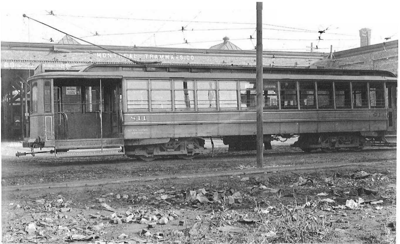
Number 940 was indeed successful and 90 more were built, numbered 703 to 881 odd numbers. The long platform is clearly shown in this view of 811 at Hochelaga barn in 1913. M.U.C.T.C. collection, C.R.H.A.
