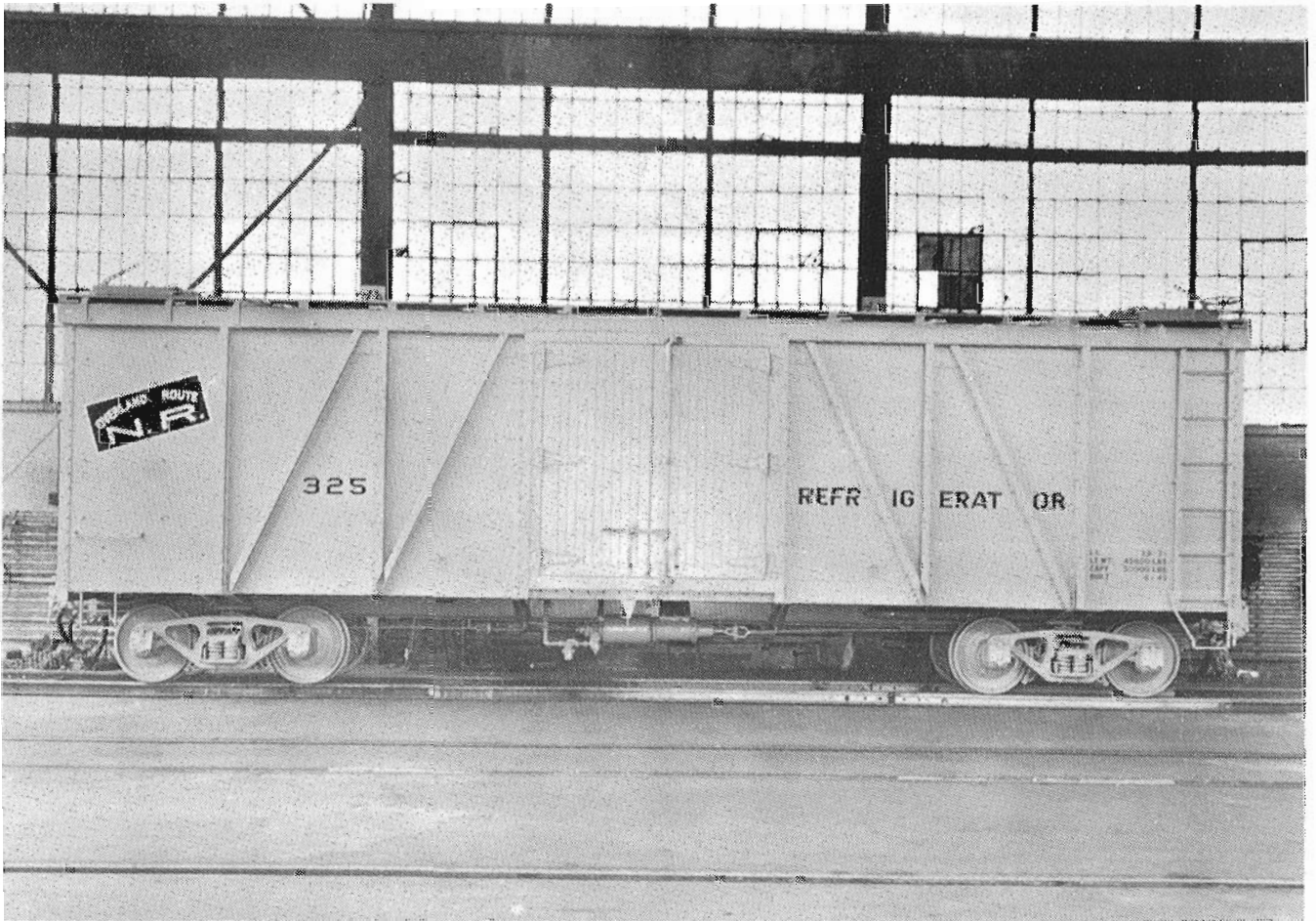
A refrigerator car for the Newfoundland Railway photographed new at the Canadian Car and Foundry shops in Montreal in June 1945. Note that it is standing on the 3'6" gauge version of "snap track".
