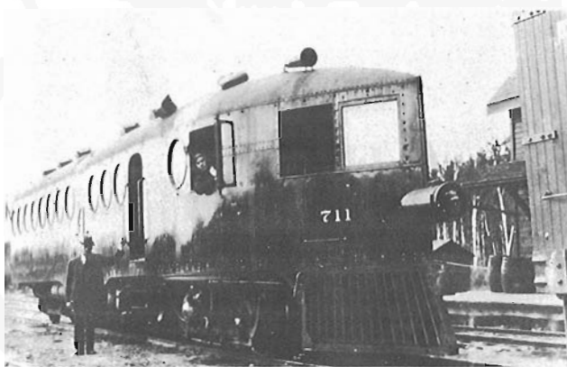
McKean car No. 711 operated on the A. & G.W. and L. & N.W. Railways. It was built by McKean in 1911 for the Woodstock & Sycamore Traction Co. It had a 55 foot long steel body and a 200 horsepower engine. This car had a seating capacity of 75 persons. The front of the car resembled the bow of a ship and the windows were like portholes. Its glaring weakness was its manually actuated transmission; it is believed that had they been equipped with a modern transmission system they would have been a huge success. This car was renumbered N.A.R. No. 1951 sometime prior to 1929. Shown are engineer Hank Kelly and conductor Frank Waite.
