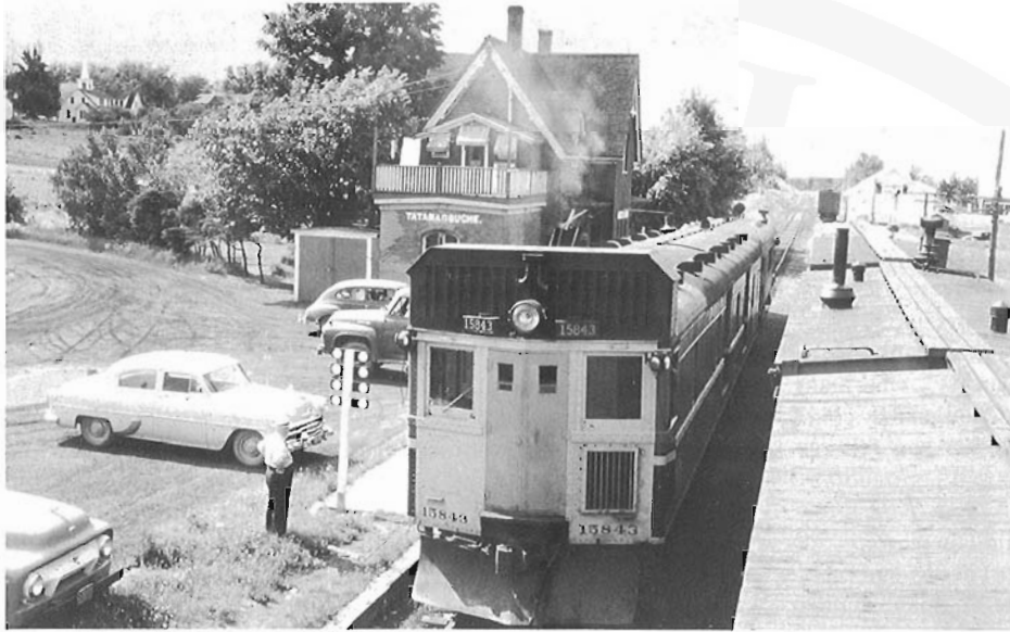
Picture 5 (five) "During the 1950's the regular passenger train on the CNR Short Line in Nova Scotia consisted of a venerable oil-electric and a lightweight trailer, the latter for passengers. Unit 15843 was built by National Steel car in 1931 for baggage- and-express service. The SpC was powered by a 300 h.p. Beardmore engine. This view, taken on 3 July 1956, shows the train at the Tatamagouche Station for what was one of the last trips for CNR. unit 15843."
