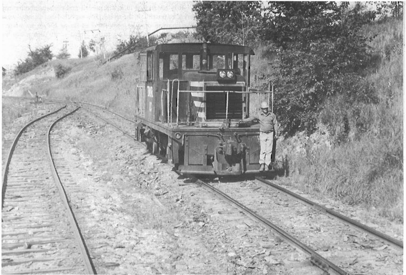
G.E. 50-tonner No. 10 (5132), originally Singer Manufacturing (New Jersey) No. 1, is seen moving along the tracks at the back of the mill property where the loaded log cars used to be brought in for unloading.
