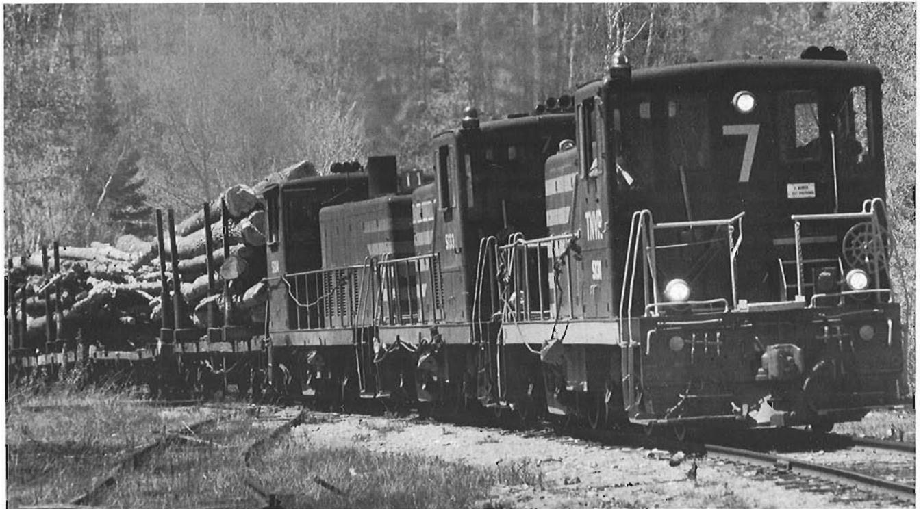
Thurso Railway G.E. 70-tonners No. 7 (5131) acquired new by the railway; No. 11 (5133) ex-C.N. 29; and No. 12 (5134) ex-C.N. 36 haul a log train south near Duhamel in May 1986.
