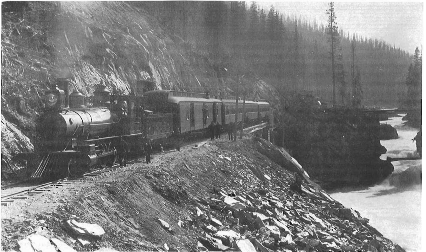
Consolidation # 402 heads up the "Atlantic Express" as it traverses the Beaver Canyon near Beaver (some 30 miles west of Golden, British Columbia) in this circa 1887 view. Behind the locomotive is a baggage-mail-express car, a first class coach, an immigrant sleeping car and a first class sleeper.
