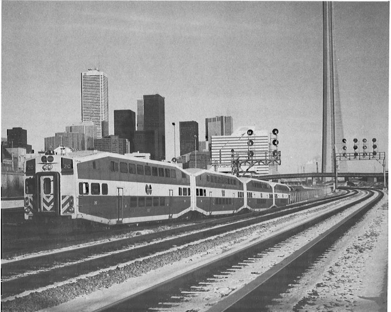
In 1983, GO Transit took delivery of 15 bi-level coaches equipped with control cabs for push-pull service. With Toronto's every changing skyline behind it, Control Car #210 emerges from the flying junction just to the east of Bathurst Street as it heads up an Oakville bound train on January 2, 1987.
