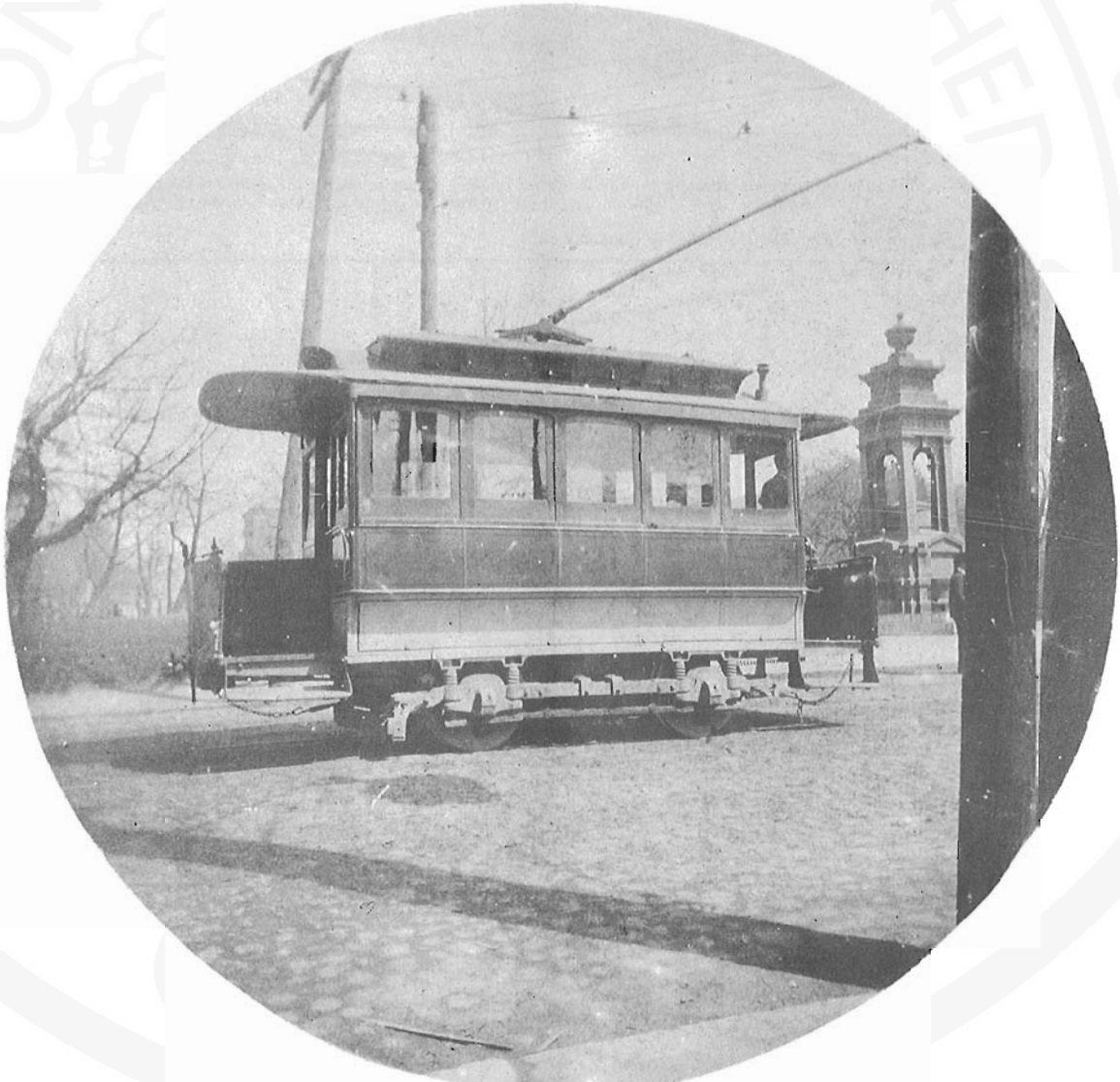
Electrification finally came in 1893 and the horses were gone by that summer. All these early electrics were, however, former horse cars, were not really suitable for electrification and did not last long. This view, taken early in 1894, shows one of the 1887 horse cars mounted on an electric truck and sporting a wooden trolley pole. Note that the car was equipped for single-ended left-handed operation.
