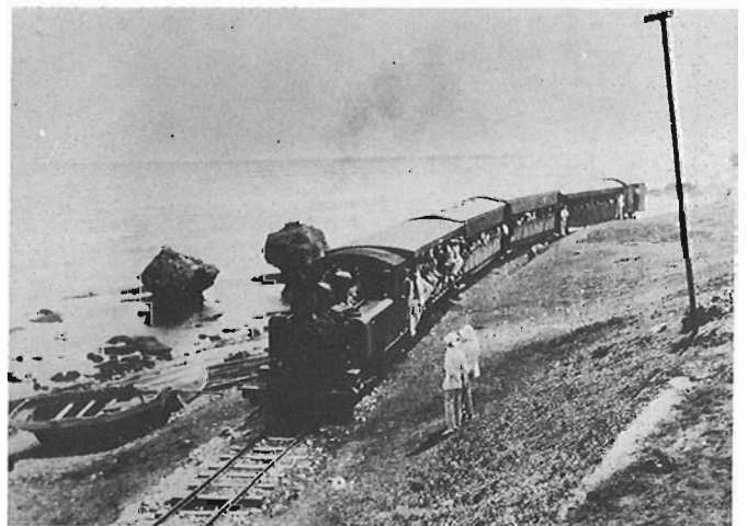
One of the Baldwin Built side tank locomotives hauling four cars and a brake van near Tent Bay in the Parish of St. Joseph circa 1920. Photo courtesy BMHS.
