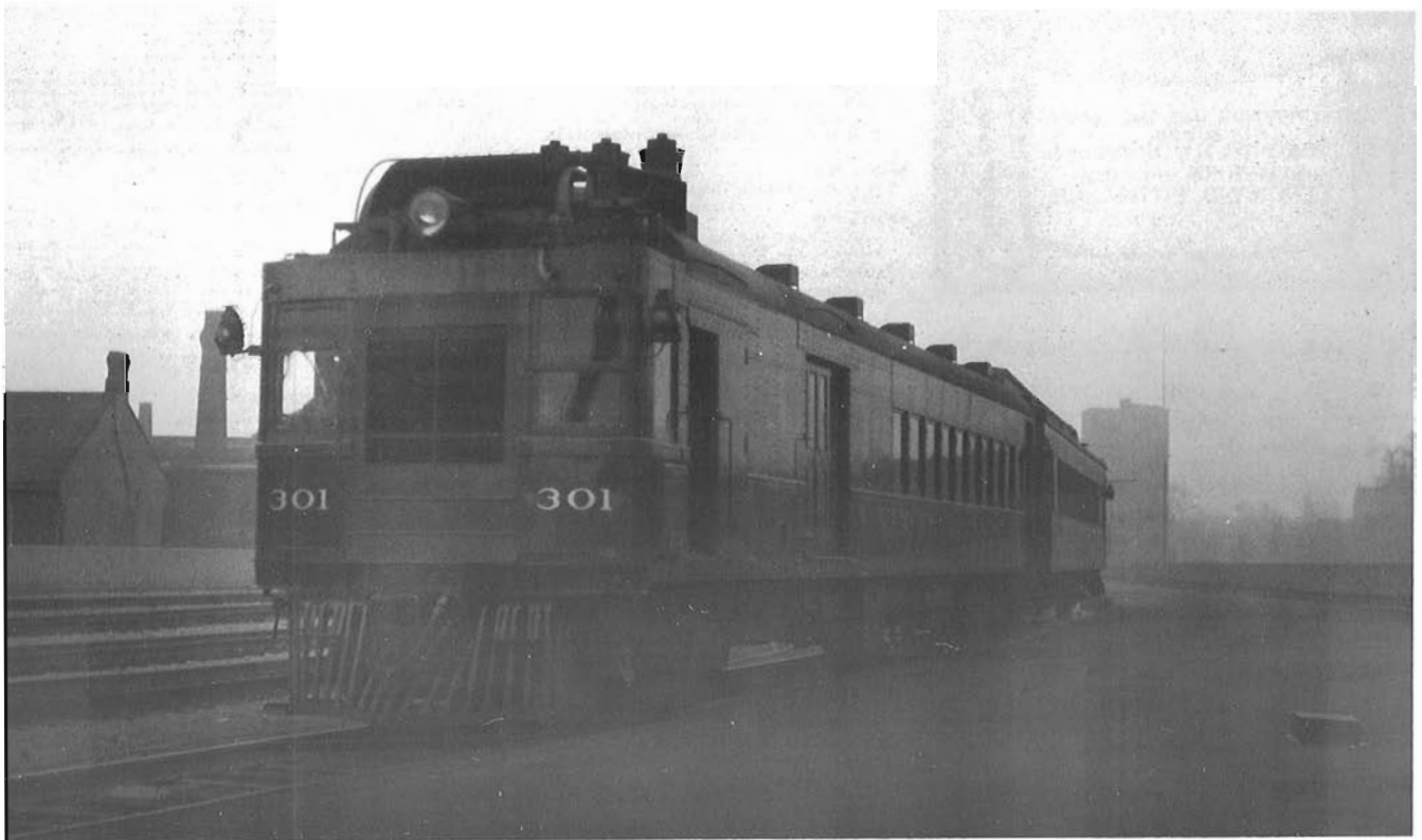
Like many North American railways during the 1920's, the TH&B bought a self-propelled car in order to reduce the cost of operating local passenger train service. Gas-electric car 301 spent most of its working life on the Welland-Hamilton-Waterford local train schedules. Pulling a wooden coach, 301 is shown departing Hamilton enroute to Welland. If all goes well, the arrival the train will arrive in Welland at 1710, one hour and ten minutes after the departure from Hamilton.
