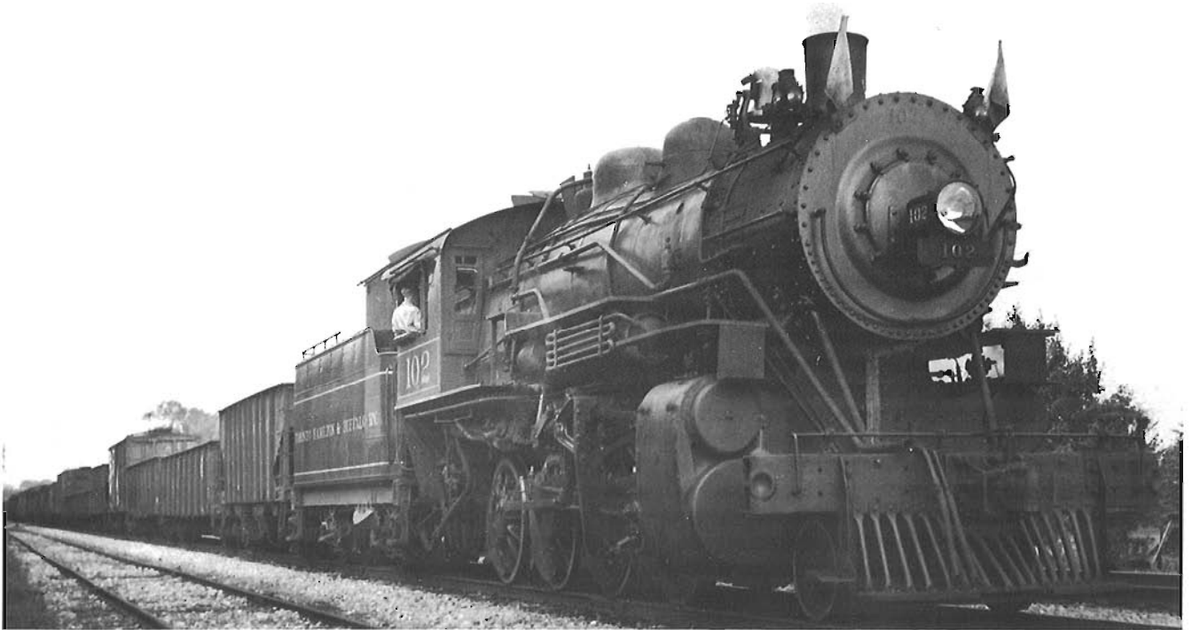
Prior to the arrival of the Berkshires, the biggest freight engines on the TH&B were 2-8-0 types. Locomotive 102 (original number 51) was built by the Montreal Locomotive Works in 1910 and could develop 45,780 pounds of tractive effort. This view taken on October 31, 1931 shows the engine on a freight train in Hamilton in a relatively unmodernized condition. Credit: Paterson-George Collection.
