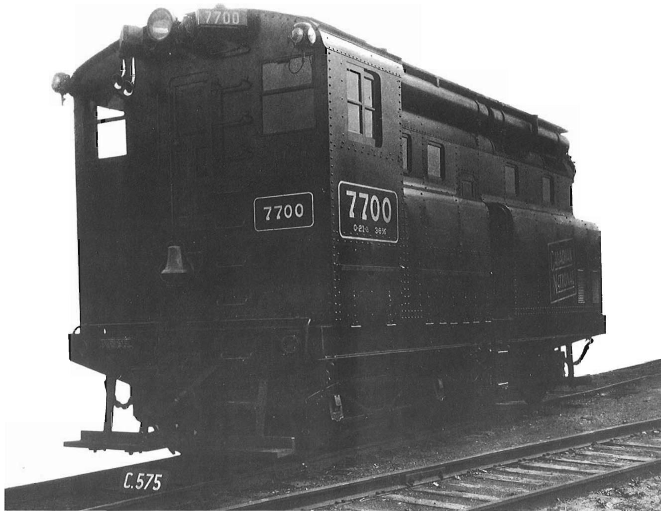
This builder's photograph shows the original paint scheme applied to the 7700. The "0-21-a" beneath the number is the CN class of this unit while the 36% is the tractive effort rating. In December 1931, CN changed the class of the 7700 to Q-1-a.
