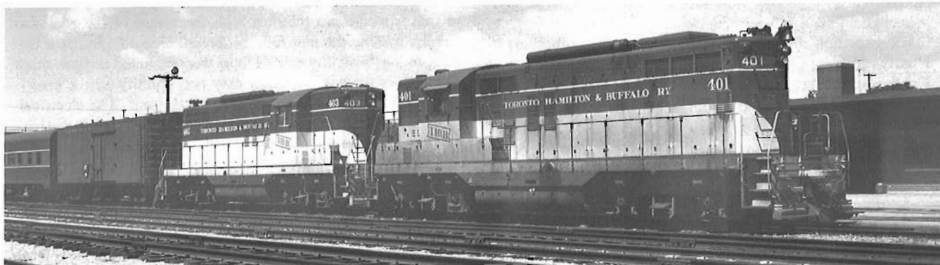
Diesels 401 and 403 head up a Buffalo bound passenger train seen here arriving at Fort Erie. The TH&B took delivery of three GP9 type diesels in 1954. Equipped with steam boilers, they permitted the retirement of the last steam locomotives on the road. Credit: National Museum of Science and Technology.
