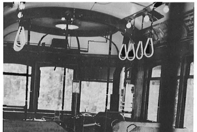
Halton County Radial Railway Museum Car 55 built in 1915, for the Toronto Civic Railways, single truck Brill, straight wood sides, arched roof, acquired by the TTC in 1921. Interior shows coal heat, rattan seats, enamel standee hand-holds. The ads proclaim the virtues of Heinz Ketchup, Wrigley's Spearmint Gum, etc.
