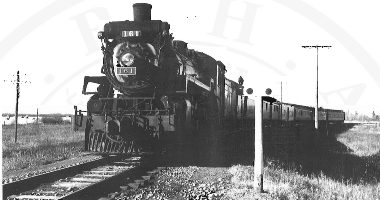
Locomotive 161 was the only Pacific type steam locomotive owned by the NAR. It was acquired from Canadian Pacific in 1947. This early 1950's view shows the southbound Train 8 from Waterways to Edmonton at Carbondale. At this time, Edmonton-Waterways train offered patrons all the amenities necessary for the overnight trip. Trailing the 161 is a wooden baggage car, a wooden mail-express car, a steel baggage car (formerly a U. S. Army troop sleeper), a wooden coach, a steel-plated diner car expected to be the car "St. John", and a steel-plated sleeper.
