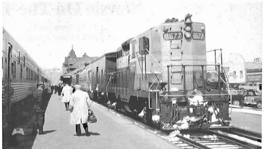
The train for Lethbridge about to leave Medicine Hat on April 30, 1967. Note that the "Dayliner" is hauled by a locomotive. This is because of an unseasonably heavy snow fall two days before. Photo by Fred Angus.
