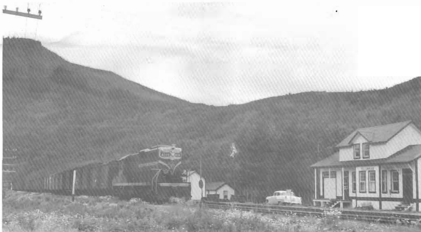
GP9 4208 leads a freight train past the station at Yellowhead, B.C. This is the first station in British Columbia when going westward. The 4208 was one of 22 GP9's General Motors delivered to CN during 1958. Canadian National photo X44384.
