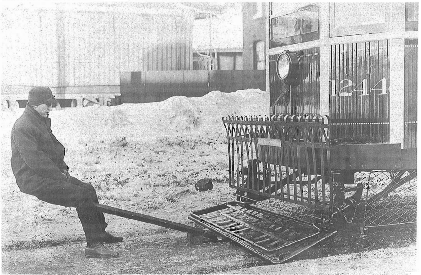
Fender "Dropped and Locked"; impossible for any object to pass under.
